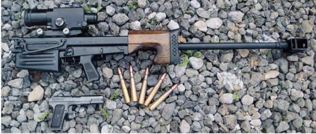
OSV-96 sniper rifle in a folded position (a version with an old muzzle break is shown) and 12.7x107 cartridges; TT pistol is placed beside it for comparison in terms of scale
